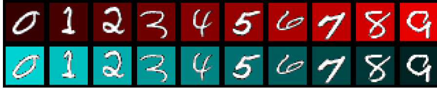
Figure 2: Colored-MNIST dataset. Top row: majority group (maroon background), digits 0–9. Background intensity increases with digit class. Bottom row: minority group (teal background), digits 0–9. Background intensity decreases with digit class. The spurious feature (background intensity) depends on the causal feature (foreground image) through the digit class, a nonlinear function of the causal feature. The ground truth label y = \mathbf{1}_{\text{digit} \geq 5} , making this a feature-mediated spurious correlation.
